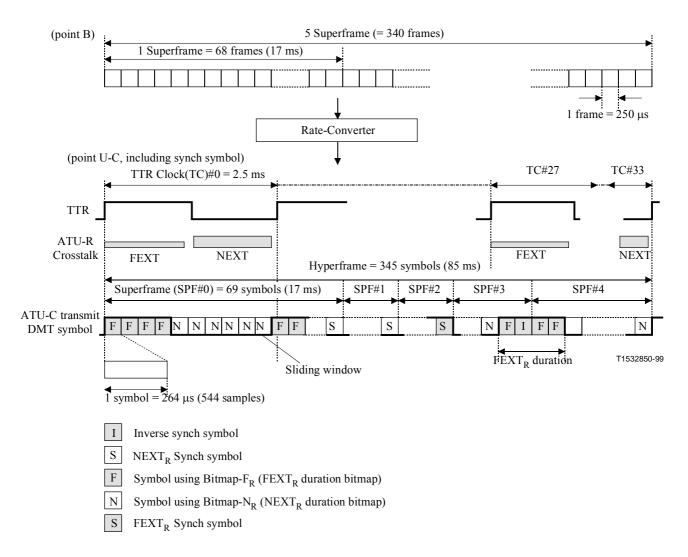
Figure Q.10/G.992.1 – Hyperframe structure for downstream
