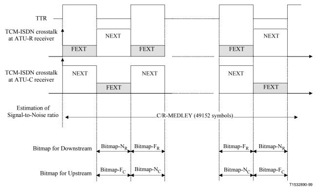
Figure Q.21/G.992.1 – Estimation of periodic Signal-to-Noise Ratio
