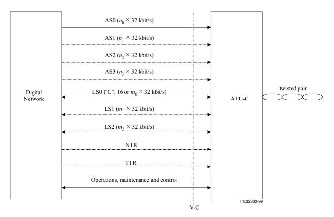
NOTE 1 – Optional bearer channels (both duplex and simplex) and features are shown with dotted lines. NOTE 2 – TTR may be generated in the ATU-C without being provided from the V-C reference point.
