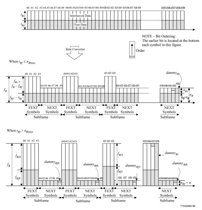
Figure Q.12/G.992.1 – Bit distribution for Rate Converter under Dual latency and Dual Bitmap mode
