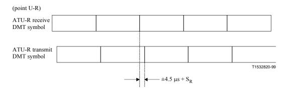
Figure Q.7/G.992.1 – Loop timing for ATU-R
