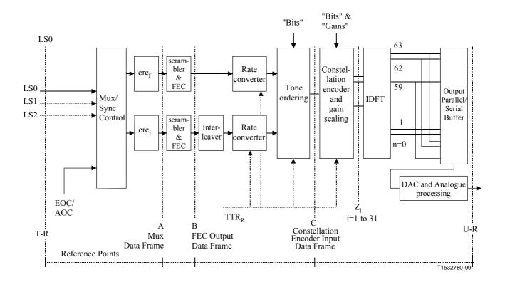
NOTE – The TTR<sub>R</sub> shall be generated in ATU-R from the received  $TTR_C$  signal, and it is locked to 690 periods of upstream sampling clock (276 kHz).
